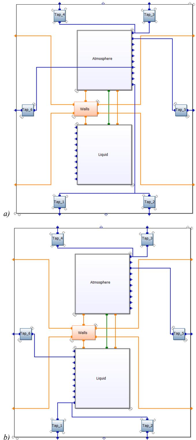
Fig. 1. Internal structure of “Tank” class with dynamic links: (a) empty tank, (b) half-filled tank.
